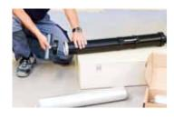
4. Allow the adhesive tube bag to slide slowly into the cylinder until it is fully inside the housing.
